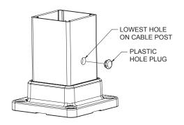
LEVEL POSTS REQUIRE SMALLER PLUGS FOR .46" DIAMETER HOLES.
